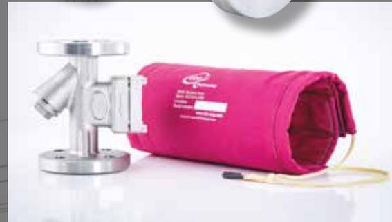
ECOFLOW differs from other Venturi orifice steam traps by incorporating the flanges into the main casting. ECOFLOWS EFK-F and EFG-F versions are both cast in one piece, in high grade Stainless Steel, which provide the traps with consistent strength, resilience and dimensional accuracy.
